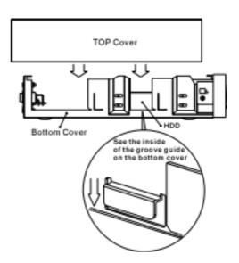
b) Slide the top cover forward until it fits tight within the front groove guide.
